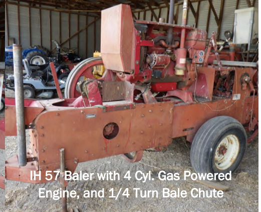
IH 57 Baler with 4 Cyl. Gas Powered Engine, and 1/4 Turn Bale Chute
