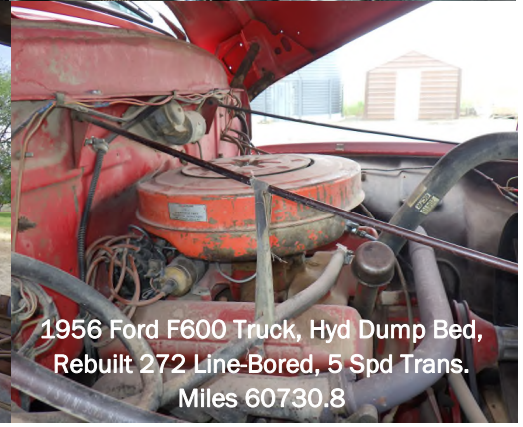
1956 Ford F600 Truck, Hyd Dump Bed, Rebuilt 272 Line-Bored, 5 Spd Trans. Miles 60730.8
