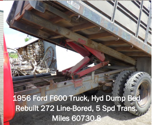
1956 Ford F600 Truck, Hyd Dump Bed, Rebuilt 272 Line-Bored, 5 Spd Trans. Miles 60730.8
